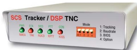
The "Tracker/**DSP** TNC" has been designed by SCS for custom applications of transferring GPS positions and other small and reappearing sets of data from e.g. remote sensors by HF or VHF radio transmission using the new SCS "Robust-Packet" modulation. Typical applications are weather stations and the tracking of vessels, cars, trucks, containers and airplanes. The unit receives the GPS data from any external NMEA device and reports it to the host station.
